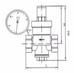
The use of direct action diaphragm structure, the internal structure is very simple, no jamming, reliable performance, durable.
