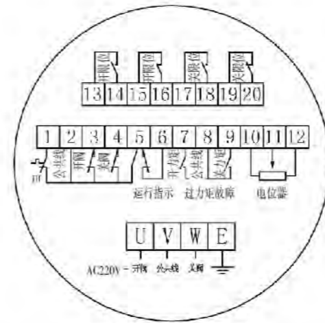
220V普通端子接线图 Wiring diagram of 220V common terminal
