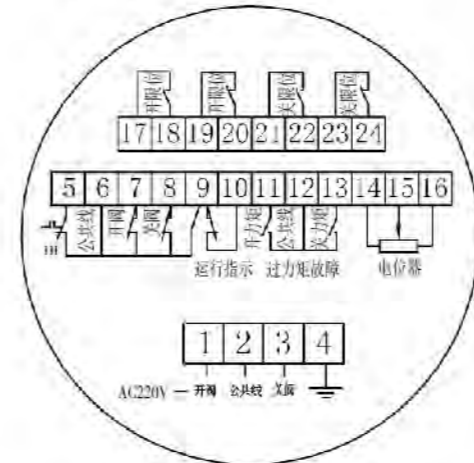
220V防爆端子接线图 Wiring diagram of 220V explosion-proof terminal
